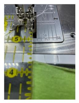
Put a ruler under your presser foot and slowly lower the needle by hand. Adjust until it is sitting directly on the ¼" line. If the edge of your ruler is not lining up with the edge of the presser foot or the ¼ " line on your throat plate, you might need to move your needle slightly to the left or right. (NB Check to make sure your throat plate will accept the new needle position.)
